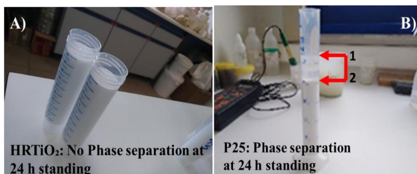
Figure 18. Dispersion and stability control by visual inspection at 24 h of a) \text{HRTiO}_2 , and b) P25 Degussa \text{TiO}_2 powder suspensions without dispersant additive
