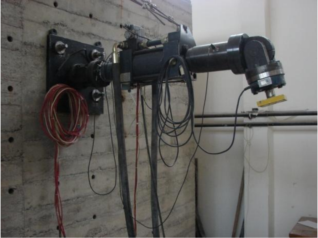
Őekil 68. Hidrolik silindir (Actuator).
