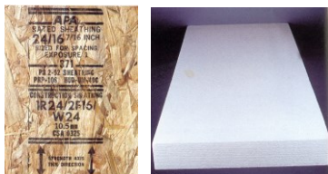
Fig. 8. OSB facings (Morley,2000) Fig. 9. EPS foam core (Morley,2000)
