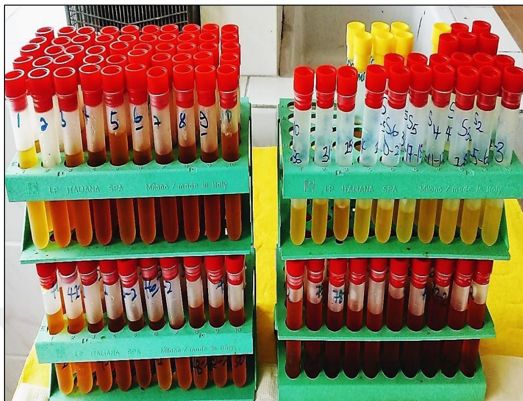
Figure 14. Filtered sample solutions ready for ICP-MS analysis of heavy metal (Photo taken by Mohammed, 2018)
