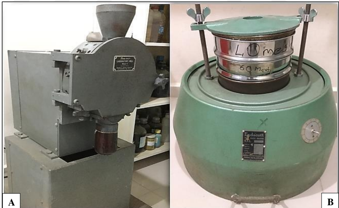
Figure 9. Thomas-Wiley's Laboratory Mill (A) and Laboratory Test Sieve Shaker (B) (Photo taken by Mohammed, 2018)
