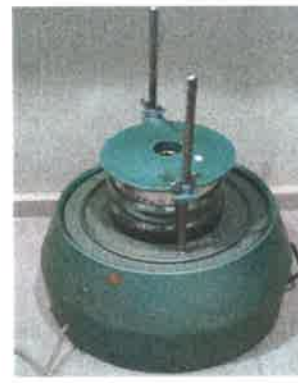
Figure 9. Wood components for WPCs preparations, (a) wood samples, (b) Thomas Milley for laboratory for wood flour preparation, (c) vibration sieve
