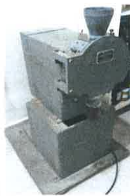
Figure 9. Wood components for WPCs preparations, (a) wood samples, (b) Thomas Milley for laboratory for wood flour preparation, (c) vibration sieve
