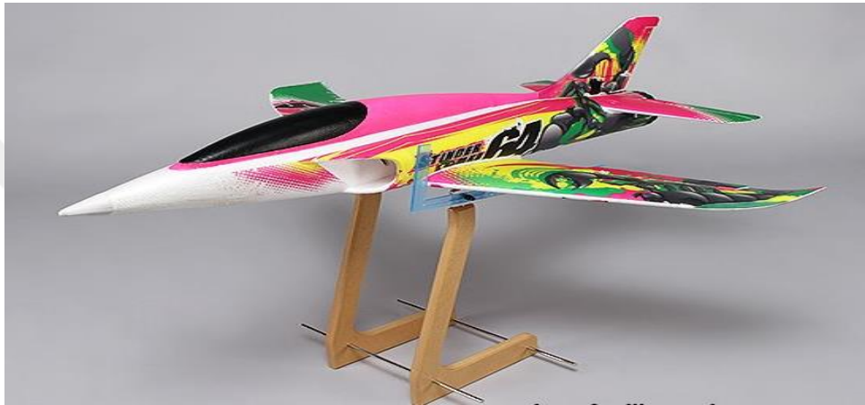
Fig. 6.9 Checking center of gravity
