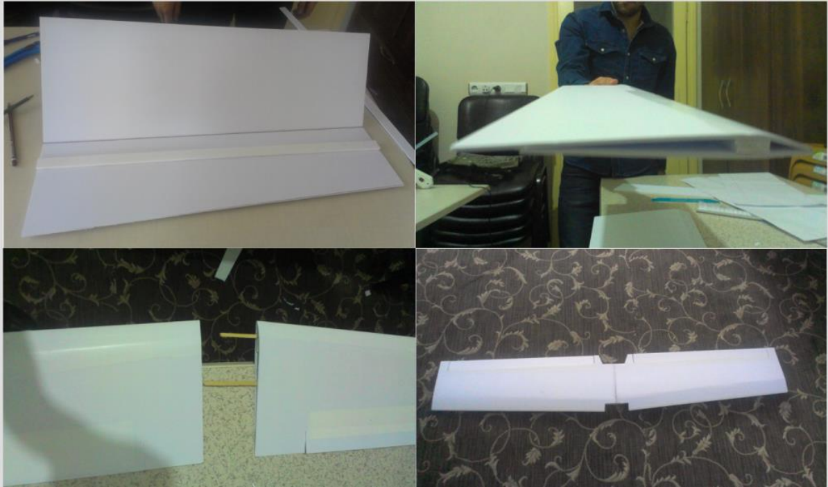
Fig. 6.4 Construction procedure of the wing
