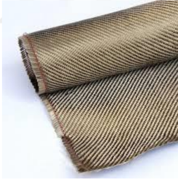
Şekil 7. Bazalt elyaf (Chikhradze et al., 2012)
