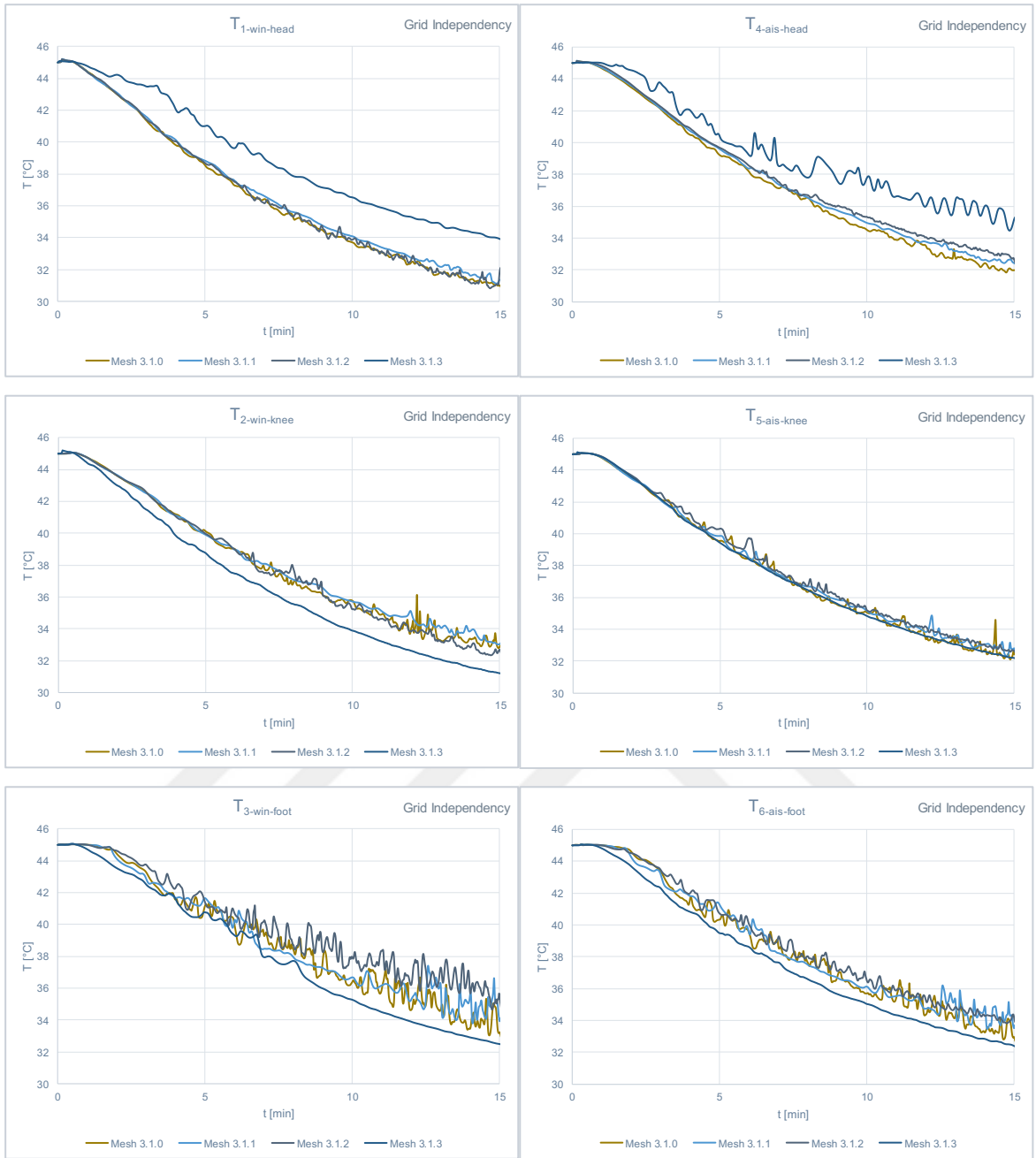
Figure 24. Temperature readings in the grid independence study
