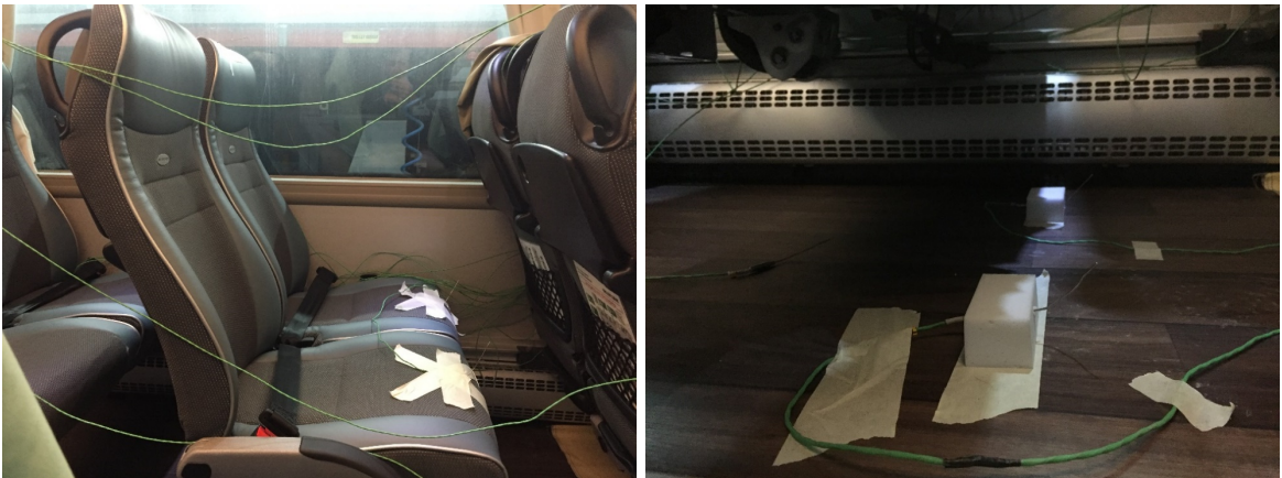
Figure 5. Thermocouple positions on the seats
