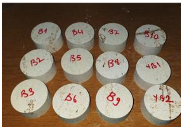
Figure 2.11. BTS test for Bayburt tuff specimens
