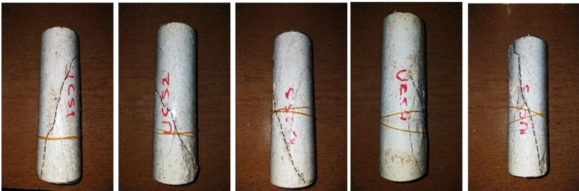
Figure 2.6. Rock specimens exhibit a shear failure with conjugates
