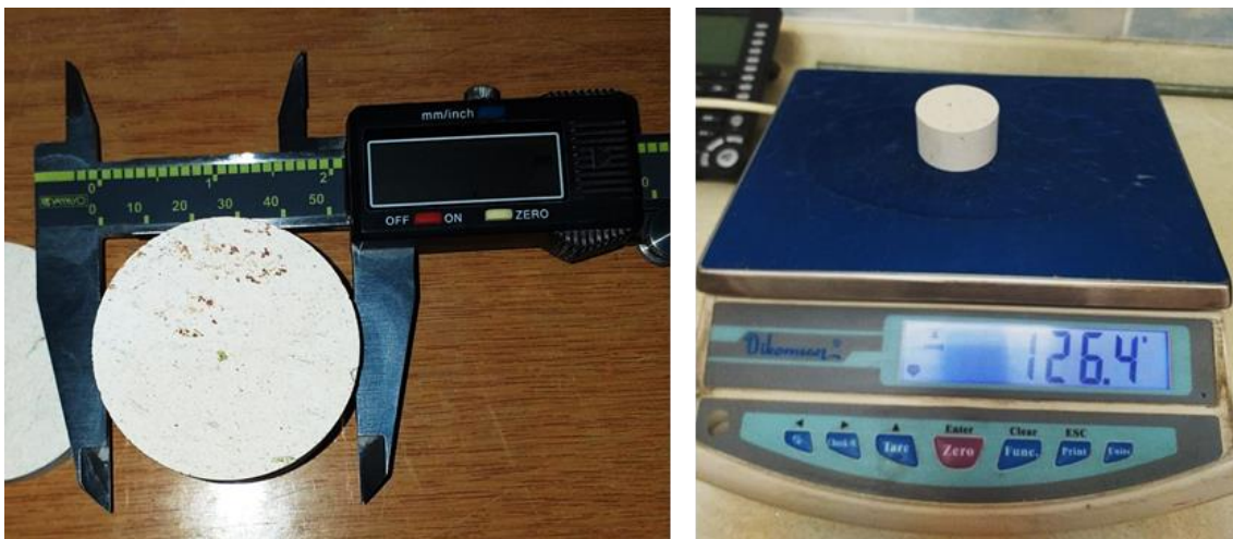
Figure 2.3. Physical measurements from Bayburt tuff specimens
