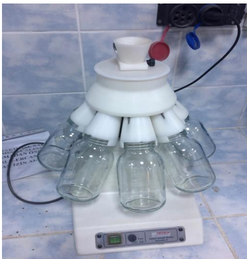
Figure 19 . Rotary sample divider (Fritsch 27)
