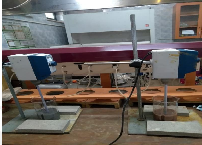
Figure 26. Experimental set up for sulphuric acid leaching tests
