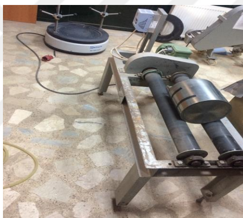
Figure 20. Rod mill used during the grinding process
