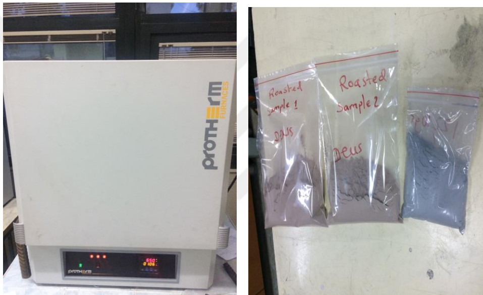
Figure 25. The Protherm furnace used in the roasting of samples as well as roasted and unroasted samples
