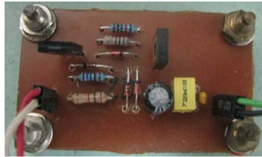
Figure A.5.4. The power supply photo chopper
