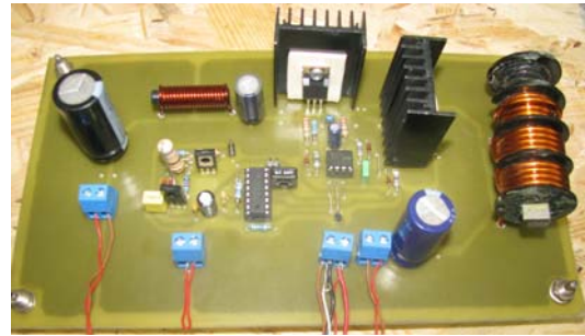
Figure A.5.2. The DC-DC buck converter general view
