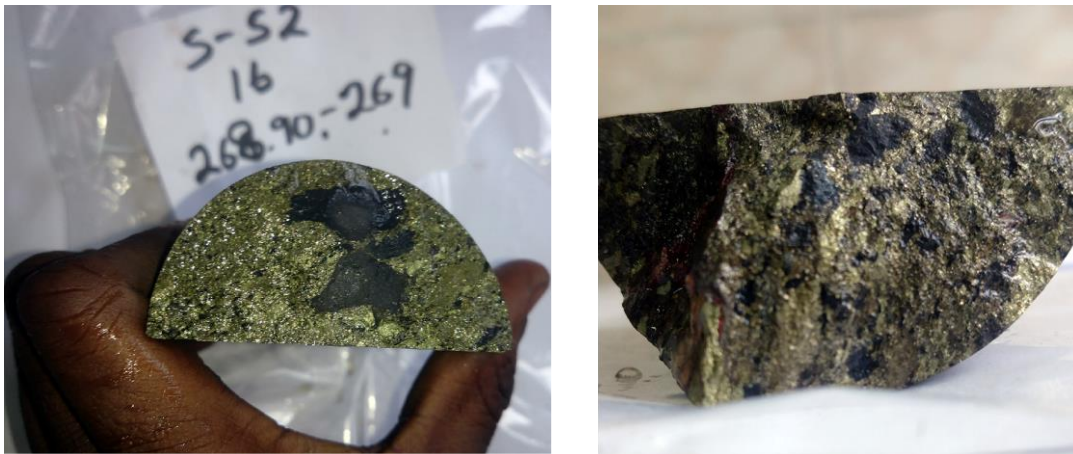
Figure 6.1. Brecciated sample of magnetite with angular fragments.
