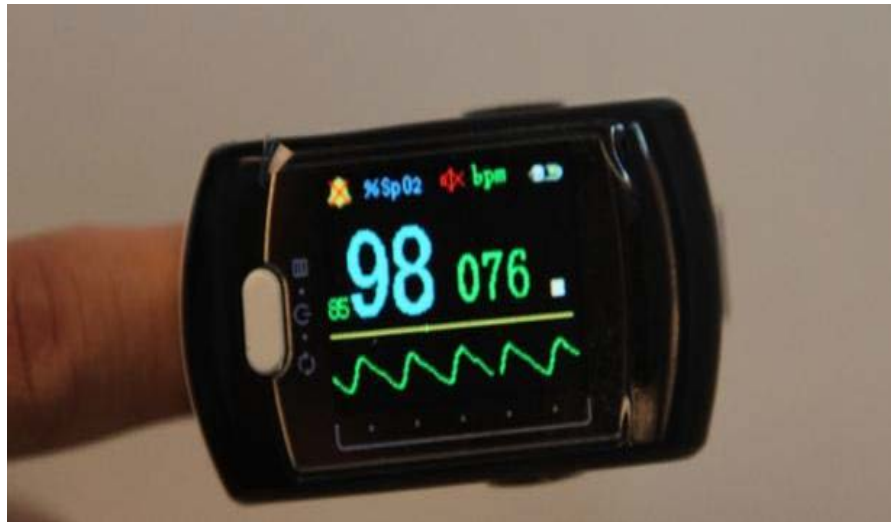
Figure 1.2. A wireless commercial finger pulse oximeter
