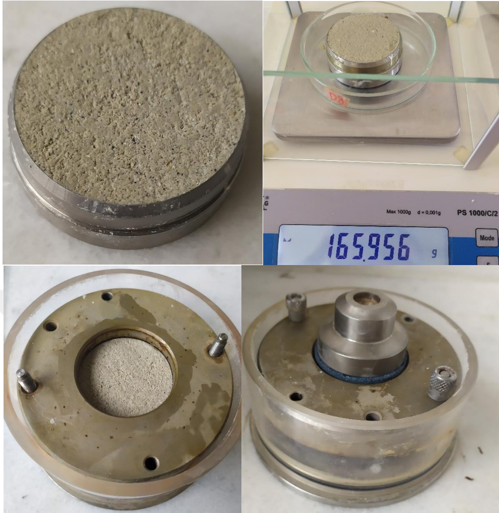
Figure 2.19. Preparation of the samples for one-dimensional swell test
